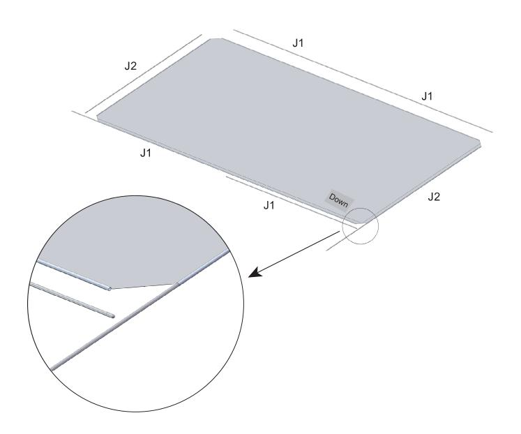
3. Thread the pull rod (N) and pull rod (M) into the screen sealing edge according to the position shown in the figure below.
