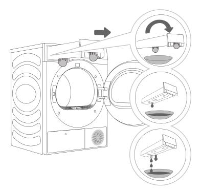
Pull out the condensate tank from the dryer (using both hands as shown in the figure), then turn it upside down over a washbasin, sink, or any suitable vessel.
