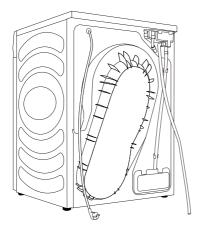
Remove discharge hose from the machine and hang it on the back.
