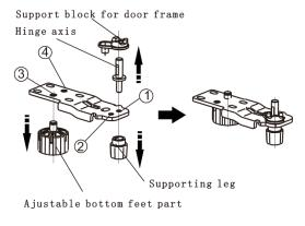
7. Set the door into its new place making sure the pin enters the bushing at the lower frame section.
