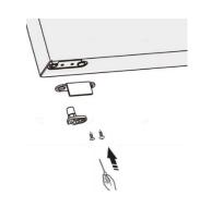
5. Place freezer flatwise, remove part ① and part ②. Loose screw ④ and then remove part ③.
