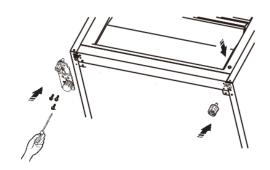
Note: 1. You need to move hinge axis from hole ① to ② , move adjustable bottom feet part from hole ③ to ④ before transfer.
