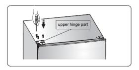
9. Put the screw hole cover and upper hinge cover ( left ) as follow diagram.
