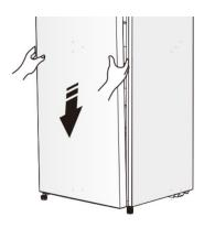
8. Replace the lid by fitting the upper hinge core into the upper door's hole, securing it with the 3 screws.
